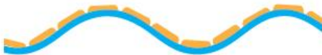
Side View: Small guard plates allow a high degree of flexibility while providing superior protection
